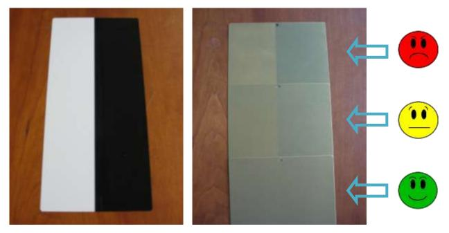
On the left, standard panel for hiding power tests. On the right, three samples of the hiding power test on the powder 6.647.0136-AJT: up to bottom, higher thickness of application.
