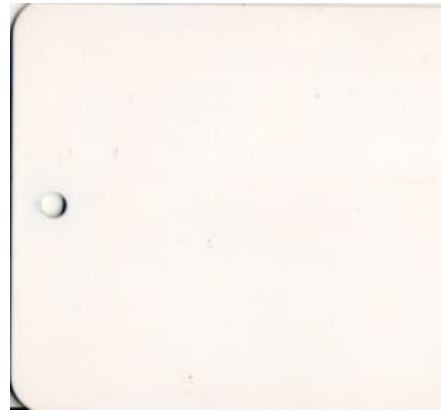
Anti-graffiti 9.445.0001-AJA (top coat on white base PE411) stained with N50 Pentel and cleaned with etasol/MEK after 10 staining/cleaning cycles \Delta E : 0,96; Residual gloss: 100%
