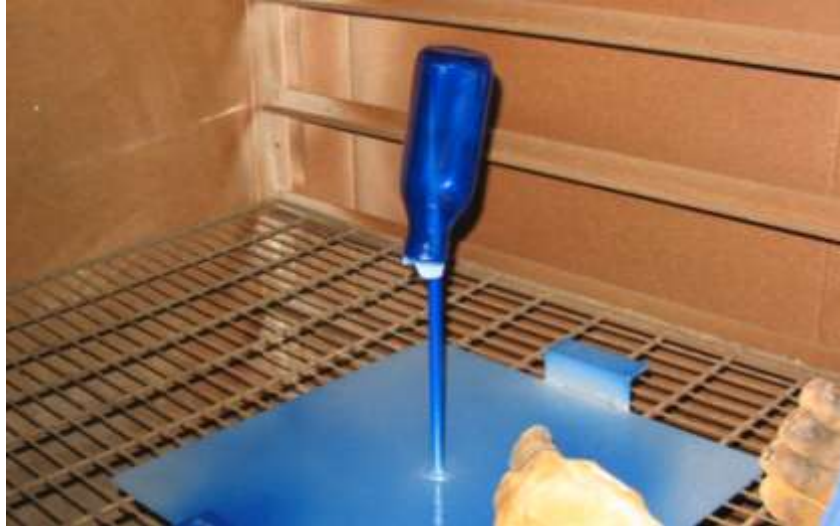
Picture 7: the sample inside the oven on its support, to complete the curing
