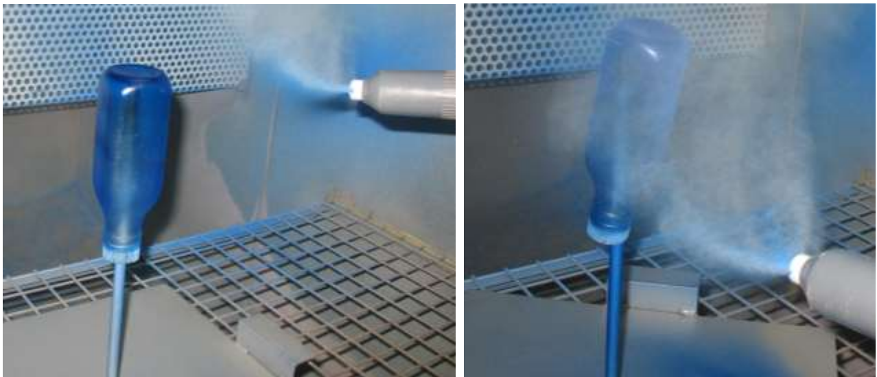
Picture 5 and 6: application of the powder-coating on the hot sample
