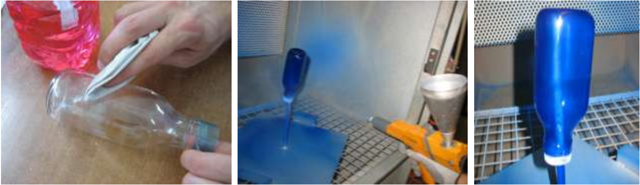
Some of the steps for the powder-coating of a glass bottle
