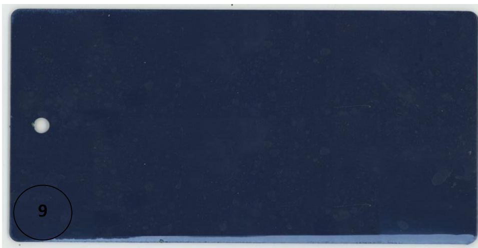
Picture 9: Sandblasted and overpainted sample panel with Ironsafe-01 after the resistance test to boiling water.
