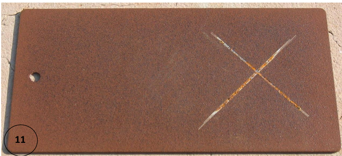
Picture 11: Sandblasted and overpainted sample panel with Ironsafe-01 after 1200 hours of test in constant climate chamber.
