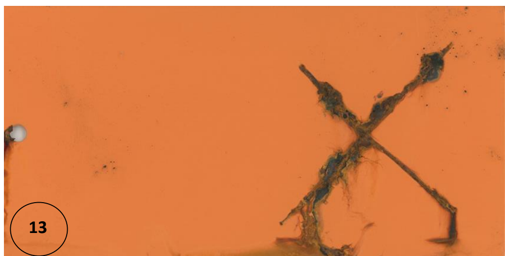
Picture 13: Sandblasted sample panel coated with Gicolor Ironsafe-01 and overpainted with polyester after 1.000 hours of exposition at NSS test
