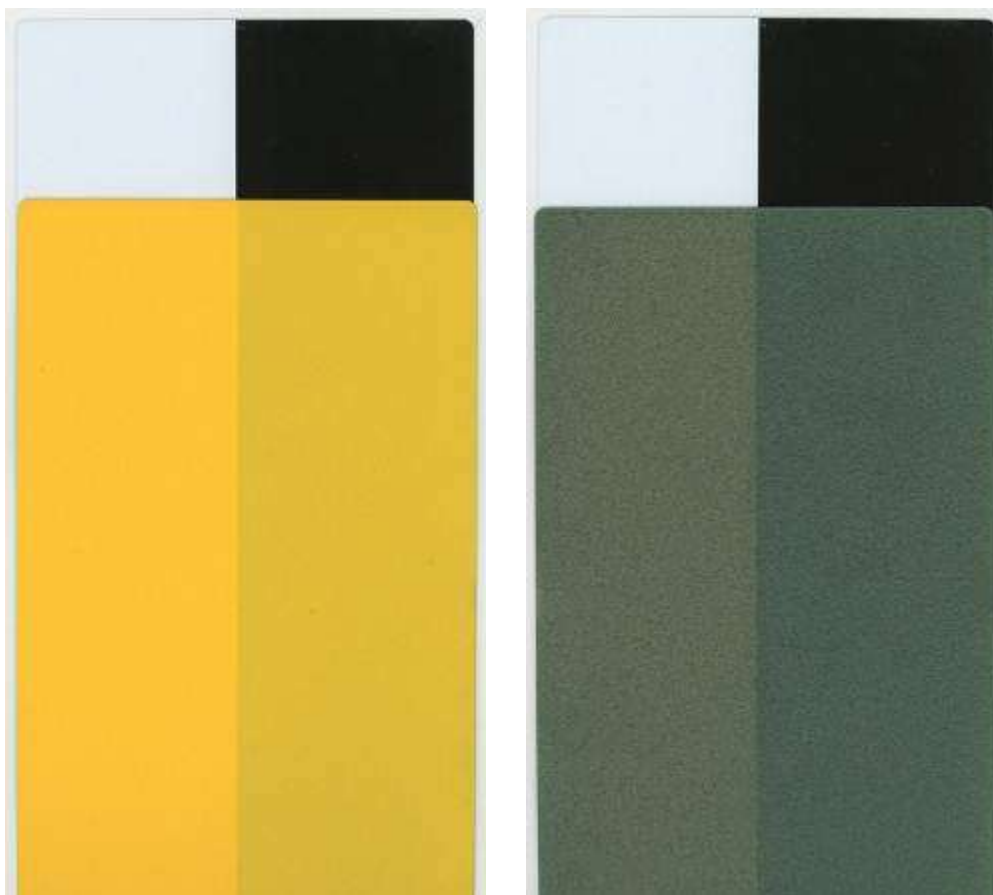
Picture 4: On the left, hiding test with Icetouch-007; on the right, hiding test which Icetouch-016.
