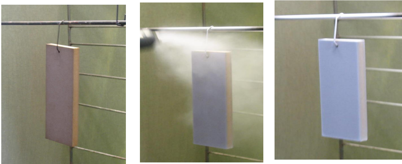
Figure 3: Example of MDF sample in the different stages of powder-coating
